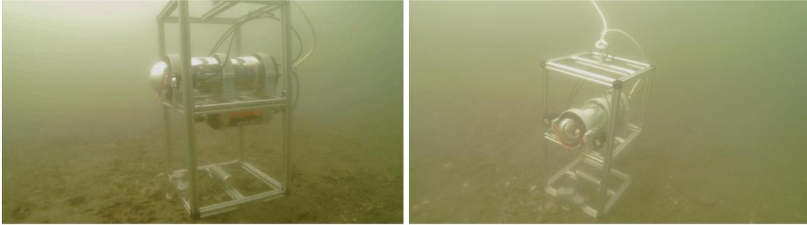
*Figure 23: Testing preliminary EMUAS prototype with mechanical wiper in Oslofjord*
