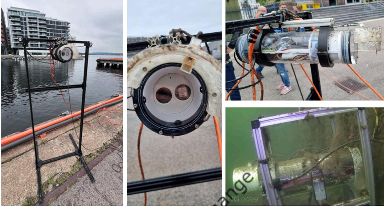
Figure 25: Testing of EMUAS camera prototype with external UV-C system, recovery after 16 days
