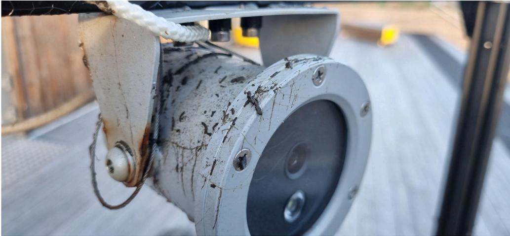
*Figure 15: Initial Linovision standalone camera system, without antifouling system*
