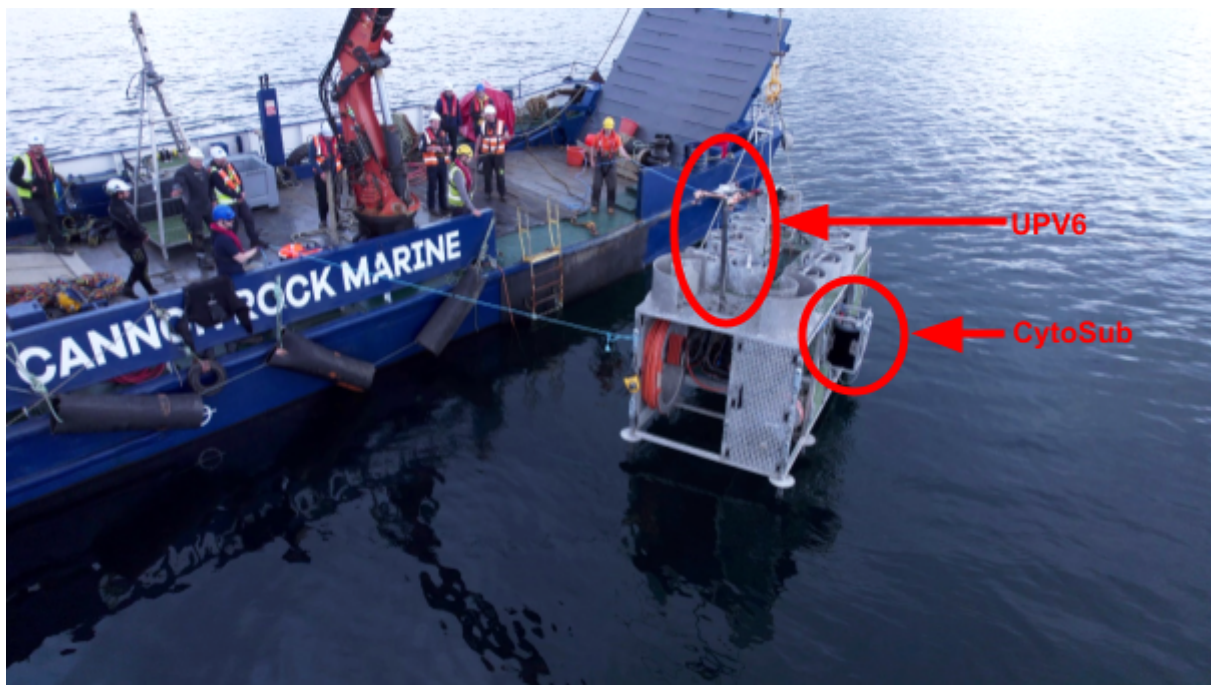
Figure 2: SmartBay being deployed as well as highlighting the location for UPV6 and CytoSub.
