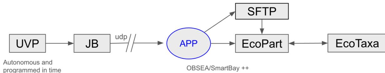
Figure 3. Schema representing the automated AIES-ZOO pipeline
