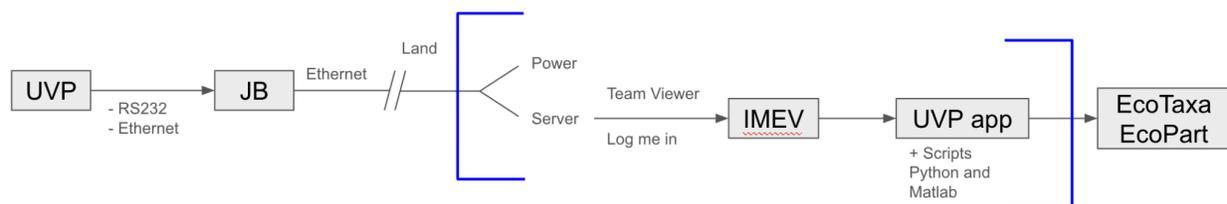
Figure 2. Schema representing the manual AIES-ZOO data pipeline
